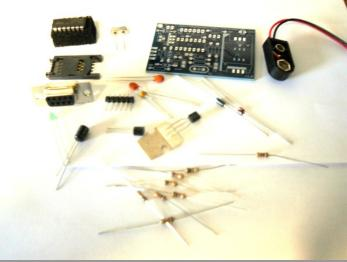
• Check to make sure you have all of the necessary parts to build the SIM card reader. You can find the list of parts under the extra guide data.
